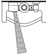
2. As the user enters the beam's effective range, 22" - 42" (559 mm-1067 mm), the object lock infrared sensor senses the user.
