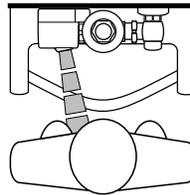
3. When the user steps away from the object lock Infrared sensor, the circuit initiates the flushing cycle to flush the fixture. The circuit then automatically resets and is ready for the next user.
