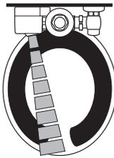
2. As the user enters the beam's effective range, 25" - 40" (635 mm-1016 mm), the beam is reflected into the scanner window to activate the Output Circuit. Once activated, the Output Circuit continues in a "hold" mode for as long as the user remains within the effective range of the sensor. If the user stays longer than 60 seconds, a full flush will automatically initiate when the user leaves,
