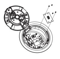
**Step 3.** Make wiring connections to AV devices and data connectors. Utilize the slots on the underside of the Evolution Series Work Surface Portal to provide strain relief for the cables.
