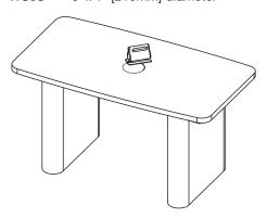
Step 2. Insert Evolution Series Work Surface Portal into opening in the table, and orient as desired.
