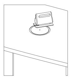
**Step 3.** Insert Evolution Series Work Surface Portal into opening in the table, and orient as desired.
