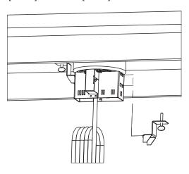
**Step 2.** Install Extron Electronics MAAP devices (Not provided) using screws provided with the devices.
