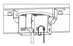
**Step 4.** If additional protection for the work surface is desired, apply adhesive-backed bumper to cover in location indicated.
