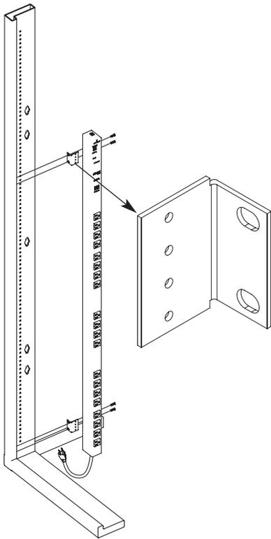
The “L” Bracket mounting option provides a simple and secure mounting solution for the SPDU20-0U.
