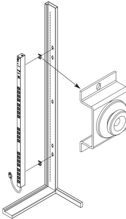
The button bracket mounting option offers a fast solution for mounting the SPDU20-0U using standard 49" [1.245m] spacing keyholes.
