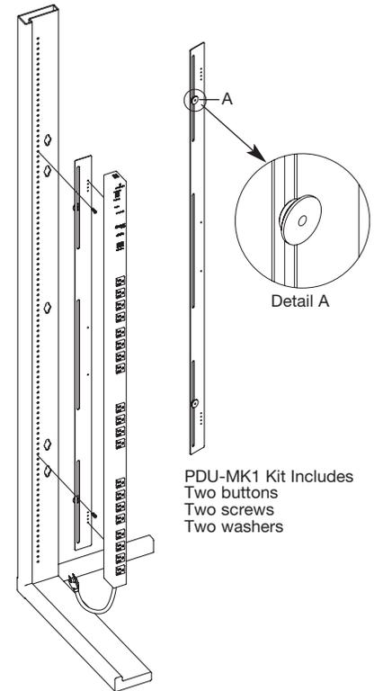
The PDU-MK1 Kit will allow you to mount the SPDU20-0U into racks and cabinets available from most major manufacturers.
