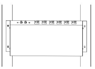
Install JPDU-A in a cabinet or 19" [483mm] rack using appropriate hardware (not provided) for mounting.
