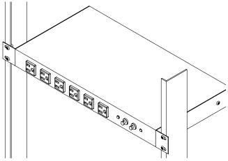
Install JPDU-A in a cabinet or 19" [483mm] rack using appropriate hardware (not provided) for mounting.
