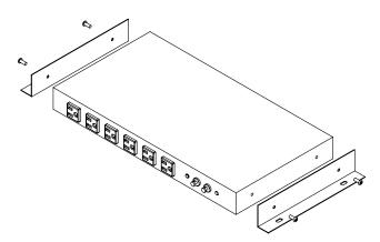
With a 5/16" nut driver, unfasten the set of 10-32 Hex head machine screws on each side of JPDU-A. Take one of the rear mounting brackets and align each side hole with the side hole on JPDU-A. Attach one rear mounting bracket using two of the unfastened 10-32 Hex screws. Repeat installations steps for the other rear mounting bracket as shown above.
