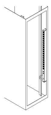
The JPDU-A has two 12 amp circuits which are indicated by the two LEDs in the front of the unit. Each circuit is protected by a 15 amp circuit breaker and 280V clamping level surge protection. A lighted LED indicates that the circuit is functioning properly and is surge protected. A non-lighted LED indicates that the circuit is not functioning properly and/or is not surge protected.
