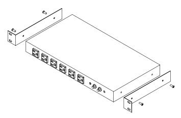
With a 5/16" nut driver, unfasten the set of 10-32 Hex head machine screws on each side of JPDU-A. Take one of the front mounting brackets and align each side hole with the side hole on JPDU-A. Attach one front mounting bracket using two of the unfastened 10-32 Hex screws. Repeat installations steps for the other front mounting bracket as shown above.
