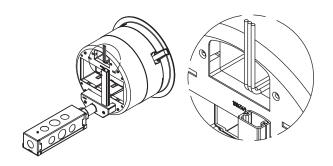
**Step 3** Slide wire tunnel out of remaining Feed Housing.
