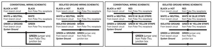
WARNING: Ground wire from junction box must be connected to system ground.
