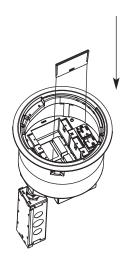
Step 2 Two dividers are provided for the bottom of the Poke Thru. Use the shorter divider on top of Wire Tunnel. Use the longer divider when separating channels without the Wire Tunnel. To install, turn divider at an angle to place inside the Feed Housing. Once inside, twist the divider to align with holes in the Feed Housing. Attach using (2) # 8-32 screws.
