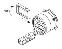
**Step 5** Reattach side Feed Housing and feed plate with (2) 8-32 screws.
