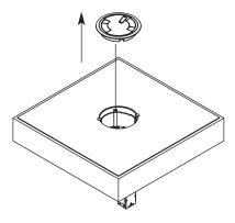
**Step 2** Remove Poke Thru from floor by bending tabs inward and pulling unit up.
