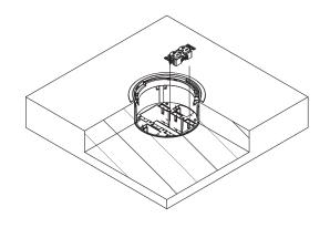
Step 2 Install plates using (2) 6-32 x 1/2" screws. (provided)
