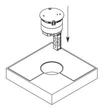
Step 2 Remove disposable plate and (2) plate clips by removing the 8-32 screws. Install Flange using the (2) 8-32 x 1/2" Cap Head screws provided with the cover assembly.
