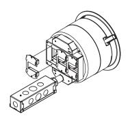
Step 2 Use (2) 8-32 screws to install new Feed Plate or housing
