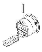
Step 4 Rotate center housing and reattach with (4) 8-32 screws.
