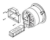
Step 2 Pull wires out of wire tunnel.
