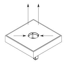
**Step 1** Remove (2) 8-32 screws and pull off Feed Plate or housing.
