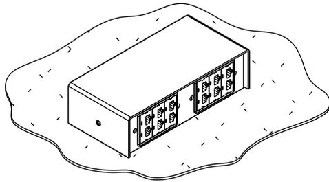
**Step 2** Remove side screws and top of 200 or 241 Service Head. Remove receptacles and communication modules. Remove cables.
