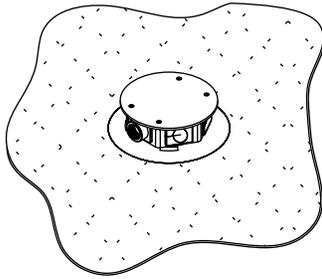
**Step 19:** Remove cables. Remove lid, eight anchoring screws, hex housing, and trim ring.
