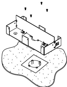
**Step 15:** Cut 6 1/2" [165mm] diameter hole in carpet that is concentric with the cored hole.
