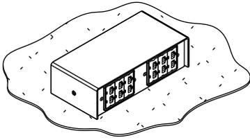
**Step 7:** Remove side screws and top of 200 or 241 Service Head. Remove receptacles and communication modules. Remove cables.
