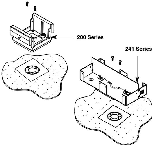
**Step 9:** Pull poke-thru device body through floor from below.
