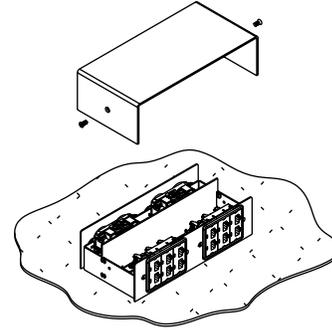
**Step 8:** Remove two anchoring screws and base of service head.
