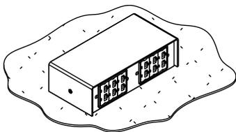
**Step 13:** Remove side screws and top of service head.
