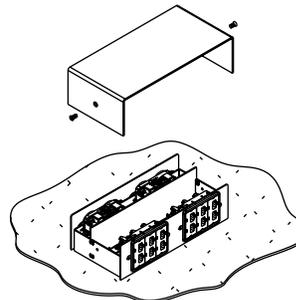
**Step 14:** Remove four anchoring screws and base of service head.
