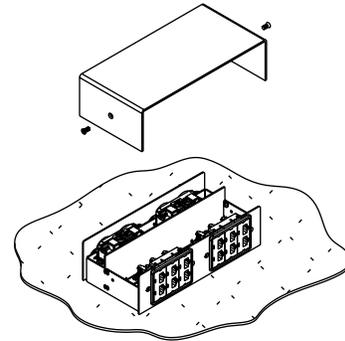
**Step 3** Remove two anchoring screws and base of service head.
