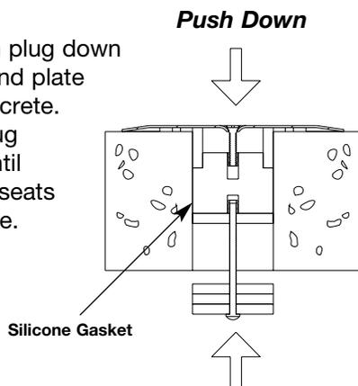
**Step 11:** Tighten screw clockwise to expand silicone gasket and complete installation on tile or carpet.
