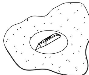
**Step 16:** Attach abandonment plate with the four #6-32 screws provided.
