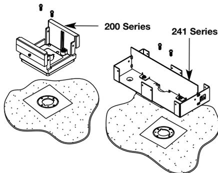
**Step 4** Attach abandonment plate with two #8-32 screws.
