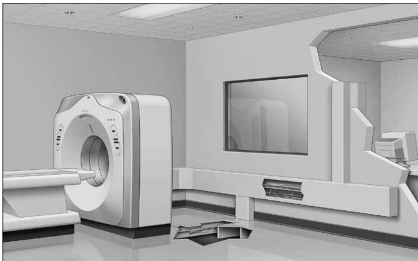
Illustration of an Aluminum Wallduct installation in an MRI Room.
