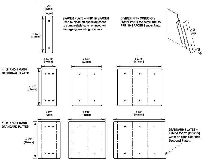
12. Determine blanking plates and spacers based on typical layouts illustrated below.
