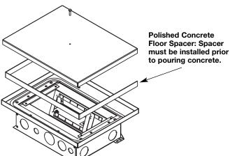
**6.** Screed to top of floor box surface. Hand troweling recommended near box edges.
