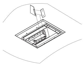
9. If tunnels are to be used, remove tunnel by removing (2) #8-32 screws. Remove the spacer plate located behind the tunnel and reinstall the tunnel.
