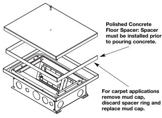
4. Remove electrical and data panels. Remove knockouts where required. Attach conduits for power and data cables using UL Listed components. All openings and unused knockouts must be closed or sealed off during final installation.
