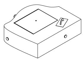
NOTE: Mud Cap is NOT a load bearing surface and additional material should be placed into the mud cap to bear the appropriate traffic loads.
