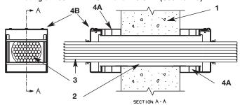
1. Wall Assembly – Min 4-1/2 in. [114 mm] thick reinforced lightweight or normal weight (100-150 pcf or 1600-2400 kg/m3) concrete for 1 and 2 hr rated assemblies. Min 6 in. [152 mm] thick reinforced lightweight or normal weight (100-150 pcf or 1600-2400 kg/m3) concrete for 3 and 4 hr rated assemblies. Wall may also be constructed of any UL Classified Concrete Blocks. Diam of opening shall be 2-1/4 in. [57 mm] or 4-3/4 in. [121 mm] for the nom 2 in. [51 mm] and 4 in. [102 mm] sleeves (Item 2).
