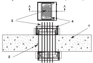
Floor & Wall Assembly – Min 4-1/2 in. [114 mm] thick reinforced lightweight or normal weight (100-150 pcf or 1600-2400 kg/m3) concrete floor or wall. Wall may also be constructed of any UL Classified Concrete Blocks\*. Maximum diameter of opening is 4-1/2 in. [114 mm].
