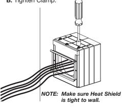
5. Move Sliding Doors to be snug around Cables by turning Side Screws.
