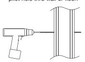
NOTE: Use core drill when going through concrete or block walls or floors.
