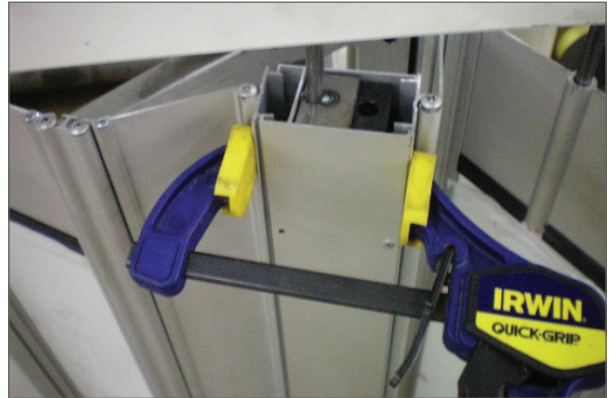
Figure 4: Use of quick clamps to join the post hinge to the post
