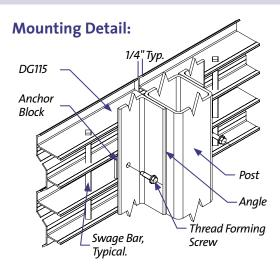
The profile and spacing of the DG115 matches standard corrugated metal sheets. This extends the sight lines of these elements in a free standing feature on the roof top of a building or at grade.
