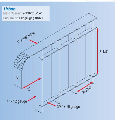
We are proud to offer our **NEW** architectural *PressLock* steel fence, ideal for multiple uses where aesthetics and security need to co-exist.
