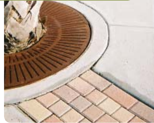
R-8738-1 • 72" x 72" 16" diameter expandable tree opening. Bolted light opening grates (10.125" x 21.75" x 5.875") for use with sub-grade lighting. 595 pounds per set. (Available without light openings, order as R-8738-2 . 568 pounds per set.)
