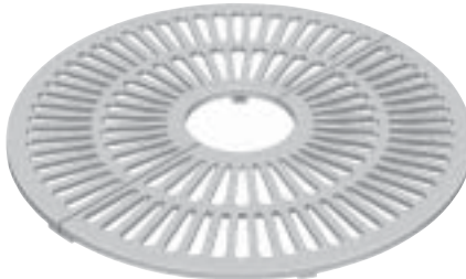
R-8833 • 50" Round 12" diameter tree opening. 266 pounds per set. Available with light opening. (Also available as 42" diameter 2-piece grate with 10" diameter expandable tree opening, order as R-8829 . 170 pounds per set.)
