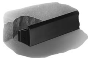
Cutaway from street, showing curb guard
