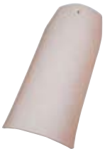
Sandstone - RB39 CRRC Product ID # 0882-0008 Solar Reflectance - 0.62 Thermal Emittance - 0.82 SRI Value - 72
