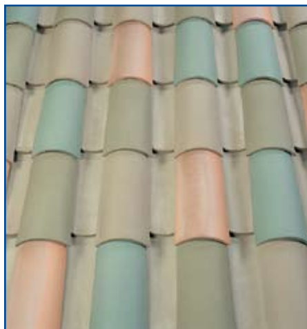
B388 Lanai Blend Solar Reflectance Avg. - 0.46 Thermal Emittance Avg. - 0.88 SRI Value - 52
