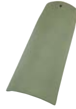
Weathered Green Medium - CC137M CRRC Product ID # 0882-0003 Solar Reflectance - 0.43 Thermal Emittance - 0.82 SRI Value - 46
