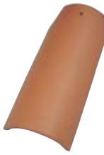
Natural Red - F40 CRRC Product ID # 0882-0030 Solar Reflectance - 0.45 Thermal Emittance - 0.88 SRI Value - 51
