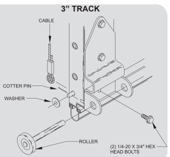
Attach lift handles in desired location on bottom retainer by using handle as a drill template. Drill (2) 1/4" holes thru section then enlarge those holes from the inside out but DON'T go thru outside skin on the door. Then assemble as shown.
