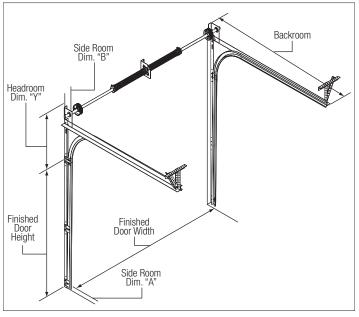
**SIDE ROOM REQUIREMENTS:** Side room is defined as the distance needed from the door opening to a wall or any obstruction.
