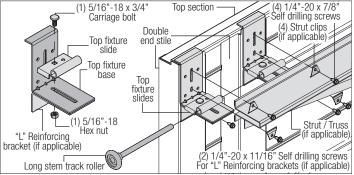
**NOTE:** If your door is to be trolley operated, it is recommended that a strut be installed along the top rail.
