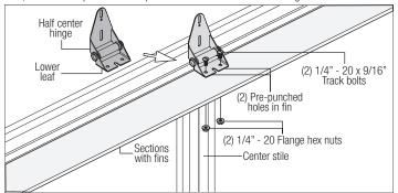
**IMPORTANT:** ONCE THE 1/4" - 20 X 7/8" SELF DRILLING SCREWS ARE SNUG AGAINST THE LOWER HINGE LEAFS, TIGHTEN AN ADDITIONAL 1/4 TO 1/2 TURN TO RECEIVE MAXIMUM DESIGN HOLDING POWER
