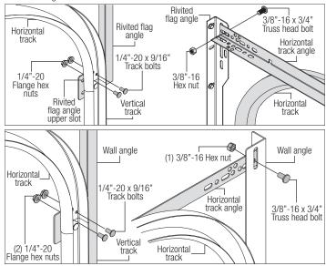
Next level the horizontal track assembly and bolt the horizontal track angle to the first encountered slot in the flag angle / angle mount using (1) 3/8" -  $16 \times 3/4$ " truss head bolt and (1) 3/8" - 16 hex nut. Repeat for other side.
