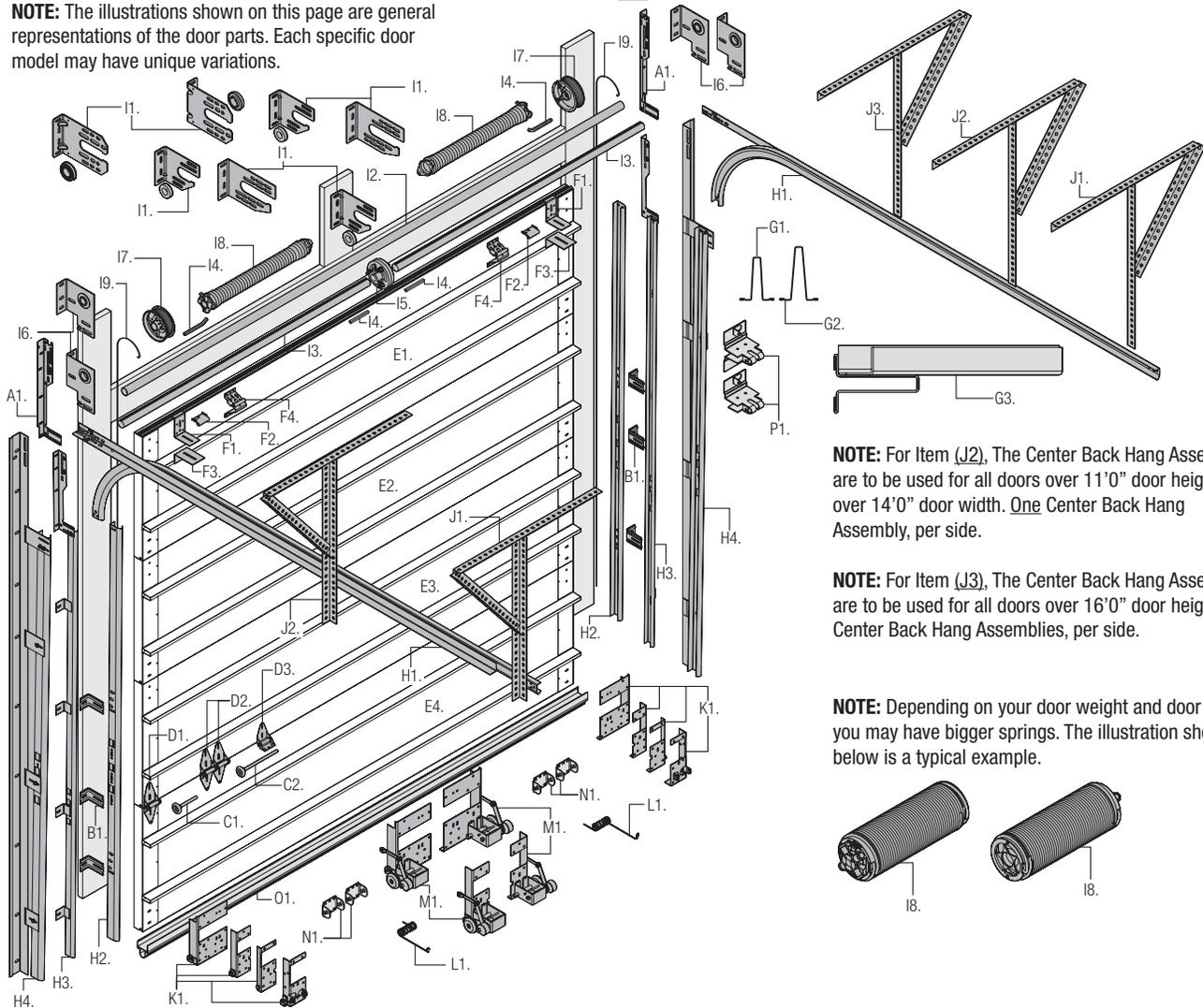
**NOTE:** For Item (J2), The Center Back Hang Assemblies are to be used for all doors over 11'0" door height and over 14'0" door width. One Center Back Hang Assembly, per side.
