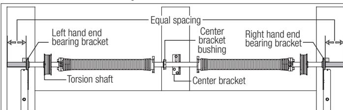
**IF YOUR DOOR HAS A COUPLER ASSEMBLY:** With assistance and starting on the left hand side of door, pick up the left hand torsion spring assembly and slide one end of the torsion keyed shaft through the end bearing bracket. Lay the other side of the torsion keyed shaft into the center bracket. Repeat the same process for the right hand torsion spring assembly. Position both torsion keyed shafts so that equal amounts of the shafts extend from each of the end bearing brackets.
