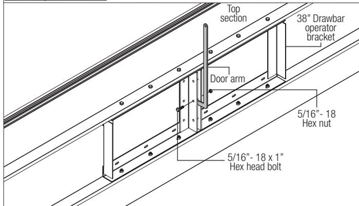
Doors over 25'2" wide and any door height, requires two 38" drawbar operator brackets.
