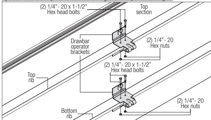
**DRAWBAR OPERATOR BRACKET (RECTANGULAR):** Locate the center of the top section
