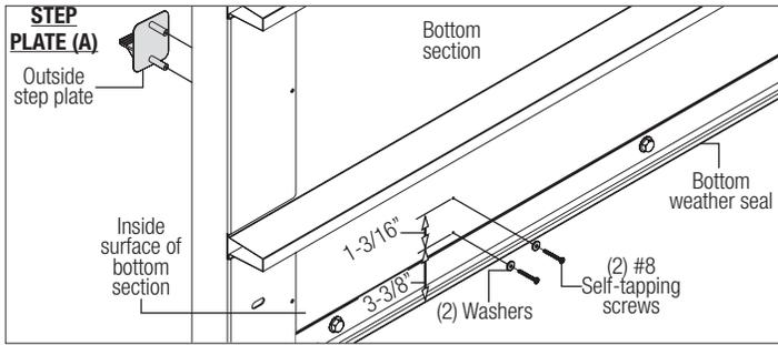
**STEP PLATE (B):** On the inside of the door, position the step plate in between the top and bottom ribs on the bottom section. Using the step plate holes as a template, mark the hole location onto the ribs of the bottom section and pre-drill (4) 3/16" dia. holes through the ribs of the bottom section.
