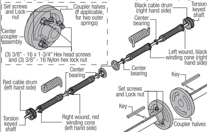
**IF YOUR DOOR DOESN'T HAVE A COUPLER ASSEMBLY:** With assistance, pick up the torsion spring assembly and slide one end of the torsion shaft / torsion keyed shaft into the center bearing. Lay the middle of the torsion shaft / torsion keyed shaft into the center bracket. Slide the other end of the torsion shaft / torsion keyed shaft into the other end bearing bracket. Position the torsion shaft / torsion keyed shaft so that equal amounts of the shaft extend from each of the end bearing brackets.
