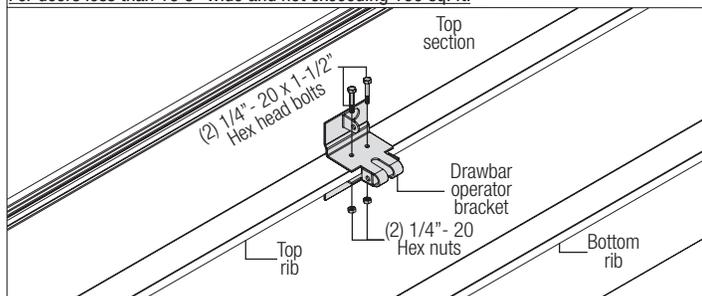
For doors over 16'2" wide through 20'2" and not exceeding 240 sq. ft., two drawbar operator brackets requires to be attached together with perforated angles.
