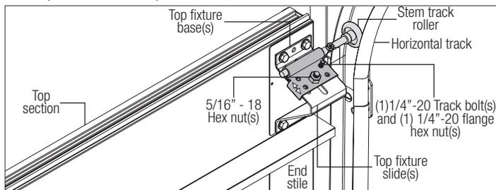
**IF YOU HAVE TOP FIXTURE BASES AND TOP FIXTURE SLIDES:** With horizontal tracks installed, you can now adjust the top fixtures. Vertically align the top section of the door with the lower sections. Once aligned, position the top fixture slide, out against the horizontal track. Maintaining the slide(s) position, tighten the (1) 5/16" - 18 hex nut(s) to secure the top fixture slide(s) to the top fixture base(s). Repeat for other side.
