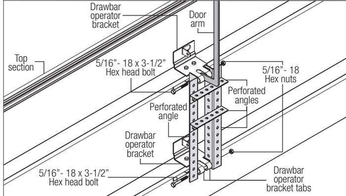
Doors over 20'2" through 25'2" wide and not exceeding 400 sq. ft., requires one 38" drawbar operator bracket.
