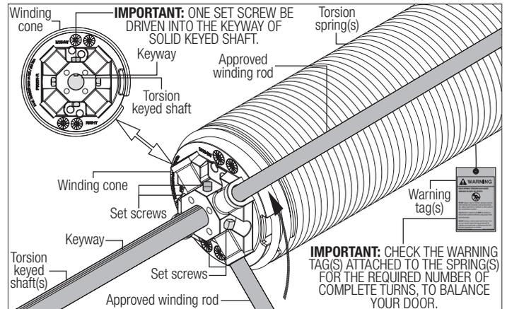
After the torsion spring is secure, use the winding rod to apply pressure in the opposite direction to ensure the set screws are securely fixed to the torsion shaft.
