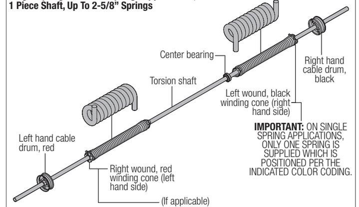
**IMPORTANT:** ON SINGLE SPRING APPLICATIONS, ONLY ONE SPRING IS SUPPLIED WHICH IS POSITIONED PER THE INDICATED COLOR CODING.
