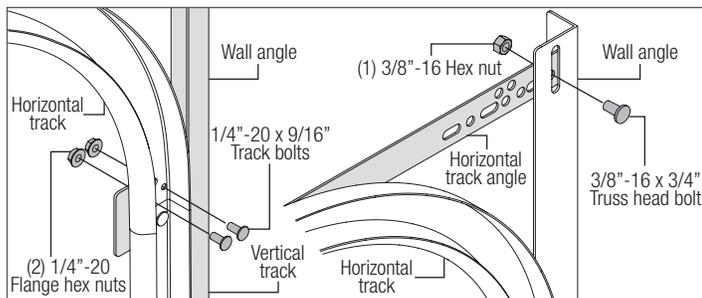
Next level the horizontal track assembly and bolt the horizontal track angle to the first encountered slot in the flag angle / angle mount using (1) 3/8" - 16 x 3/4" truss head bolt and (1) 3/8" - 16 hex nut. Repeat for other side.
