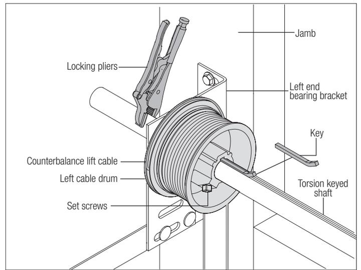
**NOTE:** Prior to securing the cable drum to the torsion shaft / torsion keyed shaft, position the cable drum tight up against the drum spacer.
