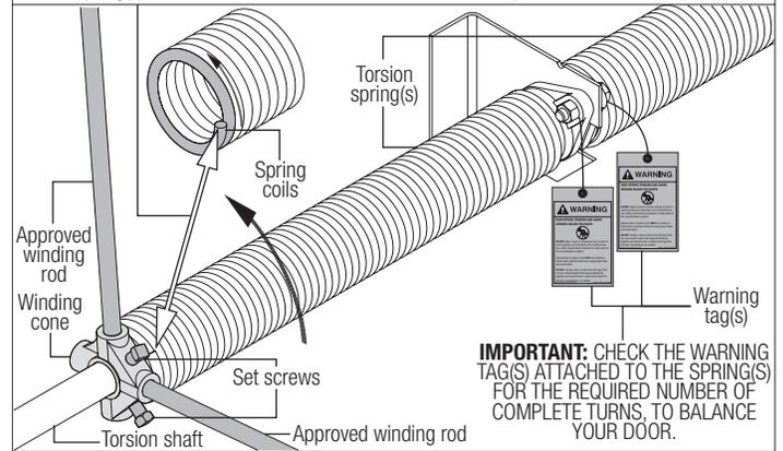
**FOR 6" AND DUPLEX SPRINGS:** Securely hold the winding rod while tightening the 4 set screws in the winding cone to 25 ft. lbs. of torque (once set screws contact the torsion keyed shaft, tighten screws 1/2 to 1 full turn).
