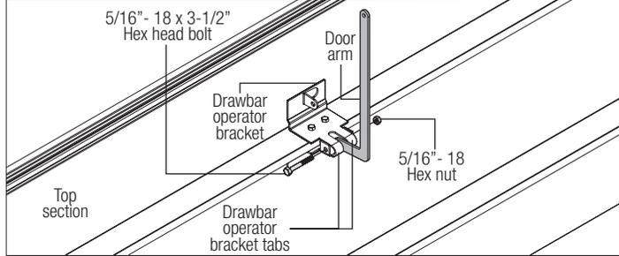
For doors over 16'2" wide through 20'2" and not exceeding 240 sq. ft., two drawbar operator brackets requires to be attached together with perforated angles.
