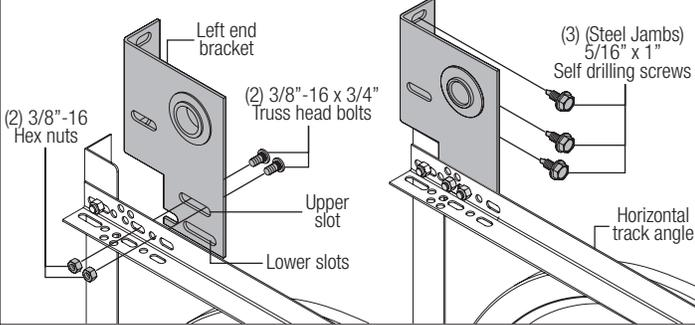
**NOTE:** This illustration shows 15" radius track with anchors to Concrete.
