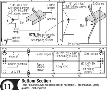
Center the bottom section in the door opening. Level the section using wooden shims (if necessary) under the bottom section. When the bottom section is leveled, temporarily hold it in place by driving a nail(s) into the jamb and bending it over the edge of the bottom section on both sides.
