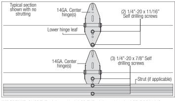
**IMPORTANT:** ONCE THE 1/4" - 20 X 7/8" OR THE 1/4" - 20 X 11/16" SELF DRILLING SCREWS ARE SNUG AGAINST THE LOWER HINGE LEAFS, TIGHTEN AN ADDITIONAL 1/4 TO 1/2 TURN TO RECEIVE MAXIMUM DESIGN HOLDING POWER.
