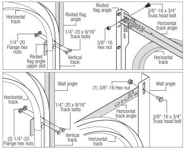
Next level the horizontal track assembly and bolt the horizontal track angle to the first encountered slot in the flag angle / angle mount using (1) 3/8" - 16 x 3/4" truss head bolt and (1) 3/8" - 16 hex nut. Repeat for other side.
