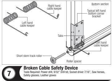
**NOTE:** If you don't have broken cable safety devices, then skip this step. Refer to Package Contents / Parts Breakdown, to determine if you have broken cable safety devices.
