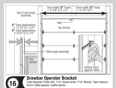
**NOTE:** If you don't have a drawbar operator bracket, then skip this step. Refer to Illustrations shown below, Package Contents or Parts Breakdown, to determine which drawbar operator bracket you have.
