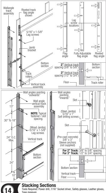
**NOTE:** Refer to door section identification, located in the pre-installation section of this manual.
