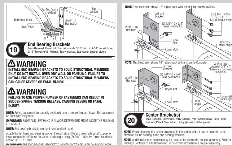
IMPORTANT: THE END BEARING BRACKET'S LOWER SLOTS ARE USED ON DOORS WITH 12" RADIUS TRACK; THE UPPER SLOTS ARE USED ON DOORS WITH 15" RADIUS TRACK.
