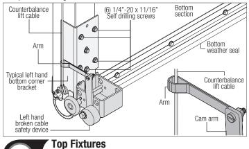
Tools Required: Power drill, 7/16" Socket driver, Saw horses, Tape measure, Safety glasses, Leather gloves
