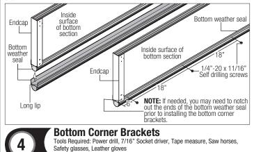
**NOTE:** Refer to door section identification, located in the pre-installation section of this manual. Refer to Package Contents / Parts Breakdown, to determine which bottom corner brackets you have received.
