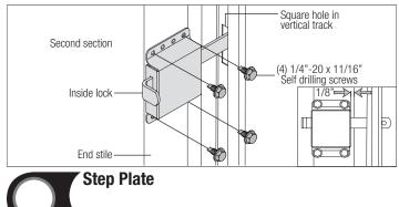
Position your step plate on the inside of the door over the bottom section endstile and on the side of the door containing the side lock. Secure the step plate to endstile using (2) 1/4" - 20 x 7/8" self-drilling screws, as shown. For doors ordered with non-keyed locks, a second step plate is provided. Install the second step plate in the same manner as the first on the lock section (second section), below the side lock.
