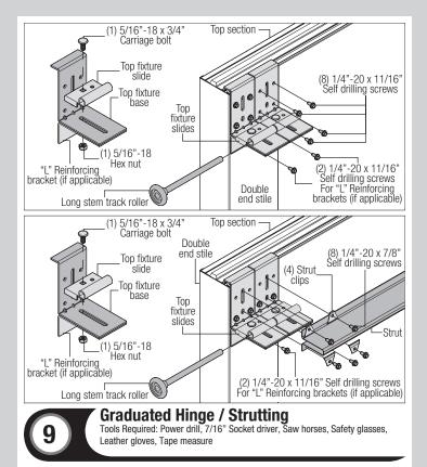
**NOTE:** Refer to the Door Section Identification, Graduated End Hinge Schedule and Strutting Schedule, to determine the appropriate hinges and or struts needed to be installed onto your section(s).
