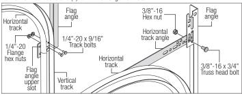
IF YOU HAVE RIVETED TRACK ASSEMBLIES OR ANGLE MOUNT VERTICAL TRACK ASSEMBLIES: To install horizontal track, place the curved end over the top roller of the top section. Align the bottom of the horizontal track with the top of the vertical track. Tighten the horizontal track to the Flag Angle / Angle Mount with (2) 1/4" - 20 x 9/16" track bolts and (2) 1/4" - 20 flange hex nuts.
