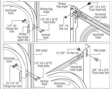
Next level the horizontal track assembly and bolt the horizontal track angle to the first en-
