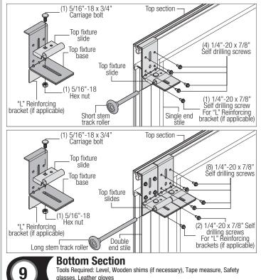
Center the bottom section in the door opening. Level the section using wooden shims (if necessary) under the bottom section. When the bottom section is leveled, temporarily hold it
