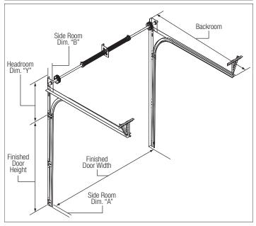
SIDE ROOM REQUIREMENTS: Side room is defined as the distance needed from the door opening to a wall or any obstruction.
