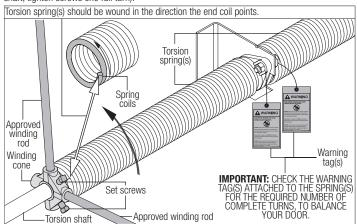
**FOR 6" AND DUPLEX SPRINGS:** Securely hold the winding rod while tightening the 4 set screws in the winding cone to 25 ft. lbs. of torque (once set screws contact the torsion keyed shaft, tighten screws 1/2 to 1 full turn).
