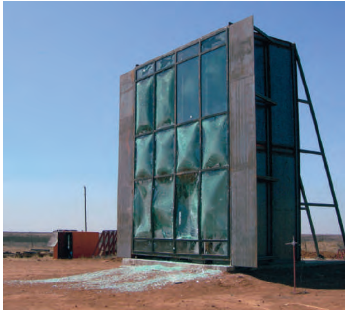
Detonation YHC 300 OG was tested in a true curtain wall application at 6psi/41 psi-ms, resulting in a GSA 3B level protection.
