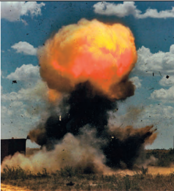
Detonation YHC 300 OG was tested in a true curtain wall application at 6psi/41 psi-ms, resulting in a GSA 3B level protection.
