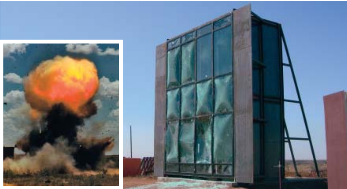
Detonation YHC 300 OG was tested in a true curtain wall application at 6psi/41 psi-ms, resulting in a GSA 3B medium level protection.
