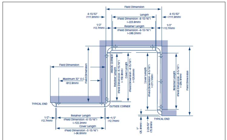
Note: If incorporating reveals at ends and corners, deduct an additional 1/4" (6.4mm) (1/8" (3.2mm) at each end) when determining cover and retainer lengths.
