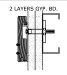
1/4"-20 X 3-1/2" BOLT AND TYPE BB TOGGLER BY MECHANICAL PLASTICS
