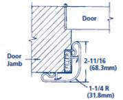
Snap precut cover in position. Cover should be lipped over one edge and pressure applied toward opposite leg from center with a "snap action" movement. Procedure should begin at bottom and be repeated as necessary for full height of cover
