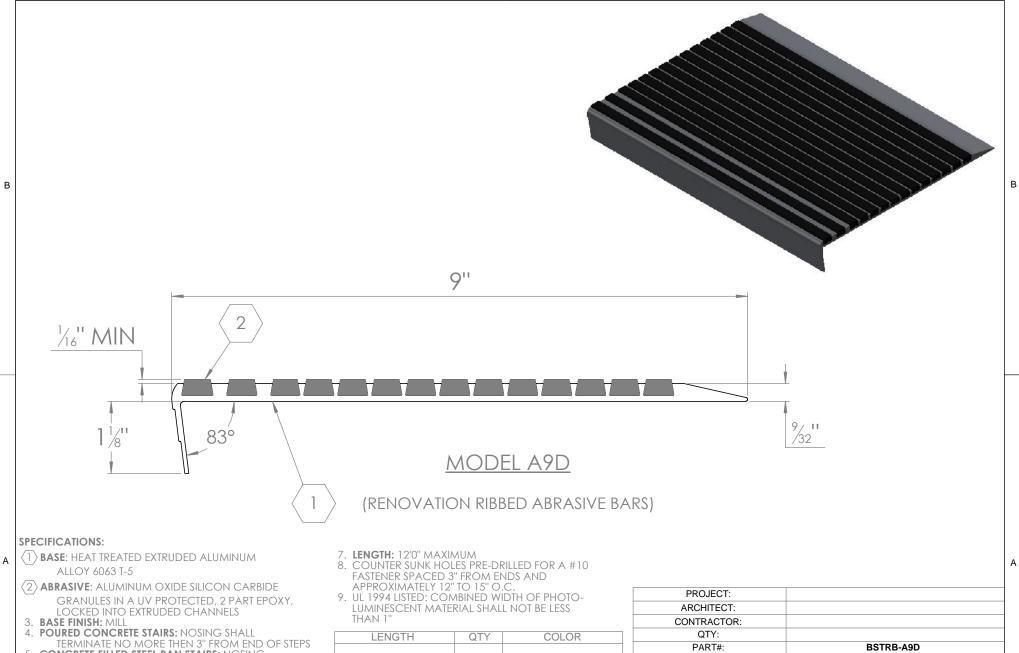
5. CONCRETE FILLED STEEL PAN STAIRS: NOSING SHALL BE FULL LENGTH OF STEPS, LESS 1/8" CLEARANCE
