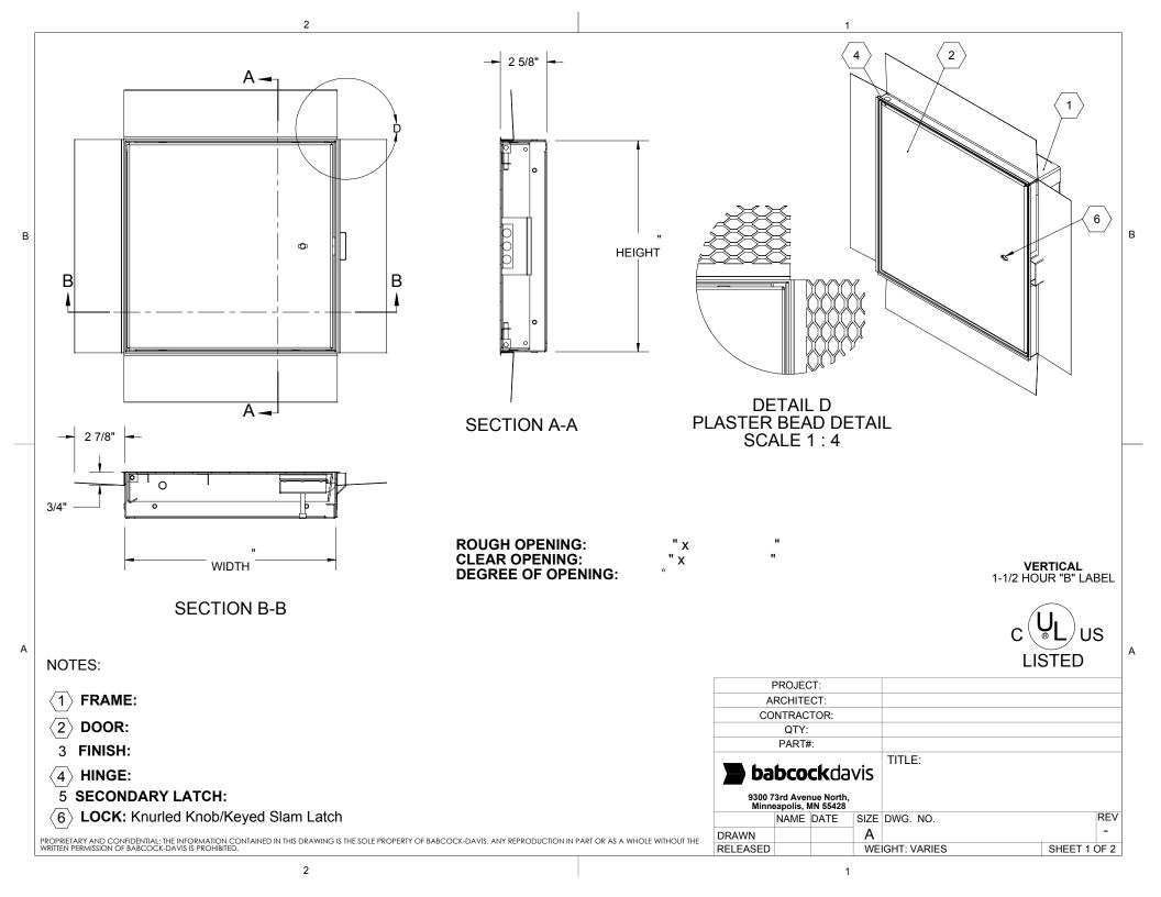
**CLEAR OPENING HEIGHT** SPRING GLIDE -CLEAR OPENING-SPRING MOUNT BRACKET **WIDTH** INTERIOR RELEASE MECHANISM -DOOR **CLEARANCE** 0 PART#: TITLE: **babcock**davis LATCH BOLT COVER EXTENDS 1/2" BEYOND OUTSIDE EDGE OF FRAME 9300 73rd Avenue North, Minneapolis, MN 55428 REV NAME DATE SIZE DWG. NO.
