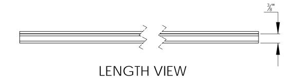
OUR OUIETFLEX ENTRANCE MATS HAVE RECYCLED LOW-DENSITY POLYETHYLENE (LDPE) HINGES AND ALL ALUMINUM RAILS. LDPE HINGES ARE QUIET AND DON'T SHRINK OR CRACK LIKE VINYL OR THERMOPLASTIC RUBBER HINGES DO. OUR ALUMINUM RAIL MATS ARE SUITABLE FOR COMMERCIAL APPLICATIONS. THEY MAINTAIN THEIR INTEGRITY IN ALL WEATHER SO THE TREADS STAY IN THE RAILS THEY ARE SUITABLE FOR COMMERCIAL APPLICATIONS.
