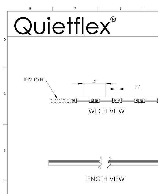
OUR OUIETFLEX ENTRANCE MATS HAVE RECYCLED LOW-DENSITY POLYETHYLENE (LDPE) HINGES AND ALL ALUMINUM RAILS. LDPE HINGES ARE QUIET AND DON'T SHRINK OR CRACK LIKE VINYL OR THERMOPLASTIC RUBBER HINGES DO. OUR ALUMINUM RAIL MATS ARE SUITABLE FOR COMMERCIAL APPLICATIONS. THEY MAINTAIN THEIR INTEGRITY IN ALL WEATHER SO THE TREADS STAY IN THE RAILS THEY ARE SUITABLE FOR COMMERCIAL APPLICATIONS.
