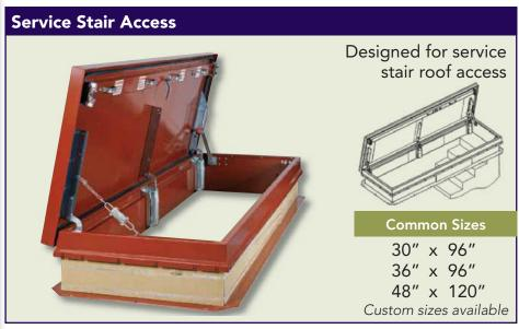
Standard roof hatches come with a 12 inch high curb, lift-assist compression springs, a locking hold open arm and a weather tight gasket seal.
