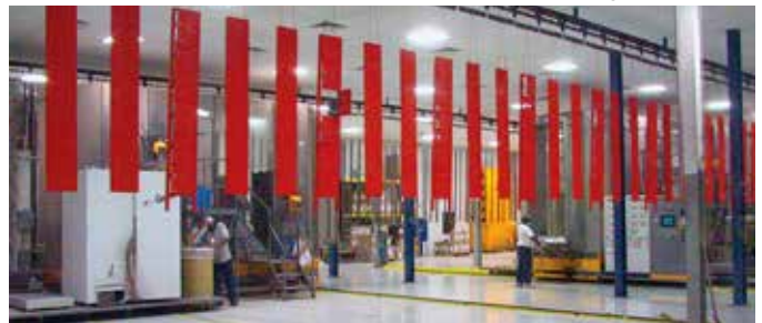
Locker components on paint line
