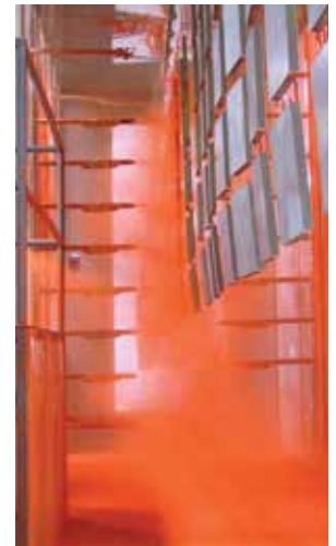
Powder coating locker parts
