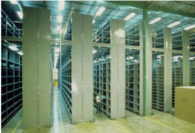
Two-level shelving with bottom serviced by picking machines.
