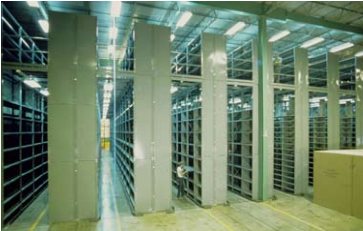
Two-level shelving with bottom serviced by picking machines.
