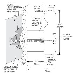
$5^{1}/_{2}$ " (140mm) height x  $1^{1}/_{2}$ " (38mm) gripping diameter, extends 3" (76mm) from the wall
