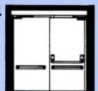
Automation to the doors is removed – latch(es) of the fire door exit hardware positively secure the door after each manual operation as intended. The doors now function as manual fire doors.
