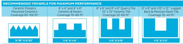
Trowel size is suggested to maximize mortar transfer/coverage. Periodically check coverage during installation. Uneven substrate may require the use of either a leveling/patching material, or larger notched trowel for proper mortar coverage.
