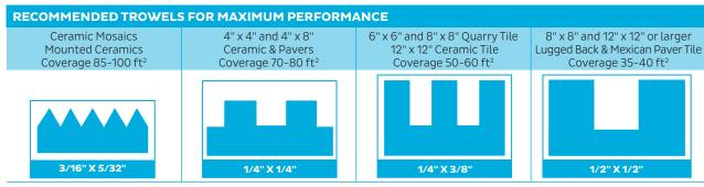
Trowel size is suggested to maximize mortar transfer/coverage. Periodically check coverage during installation. Uneven substrate may require the use of either a leveling/patching material, or larger notched trowel for proper mortar coverage.
