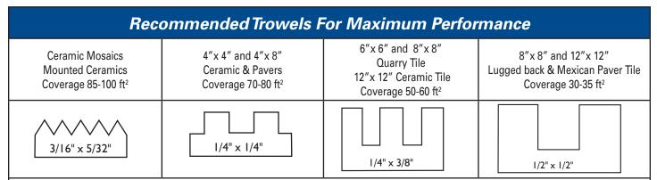
Trowels size is suggested to maximize transfer/coverage of mortar. Periodically check coverage during installation. Uneven substrate may require the use of either a leveling/ patching material, or larger notched trowel for proper coverage of mortar.
