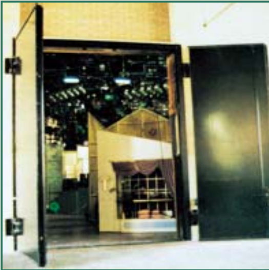
ABC STUDIOS—stages 57 & 59 – Hollywood, California Two pair of 14' wide x 18' high manually operated FSTC51 swing doors. The doors are 4" thick and weigh 4,000 pounds per leaf. The hinges are designed specifically to accommodate the leaf weight, providing for ease of manual operation.
