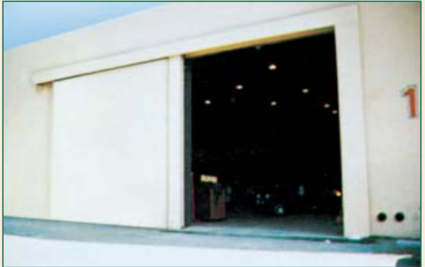
The 18' wide x 20' high, 6" thick FSTC63 side sliding concrete acoustic door weighing approximately 40,000 pounds can be designed for either interior or exterior applications. The door system is independent of the building, allowing it to be considered as a replacement door for existing doors.
