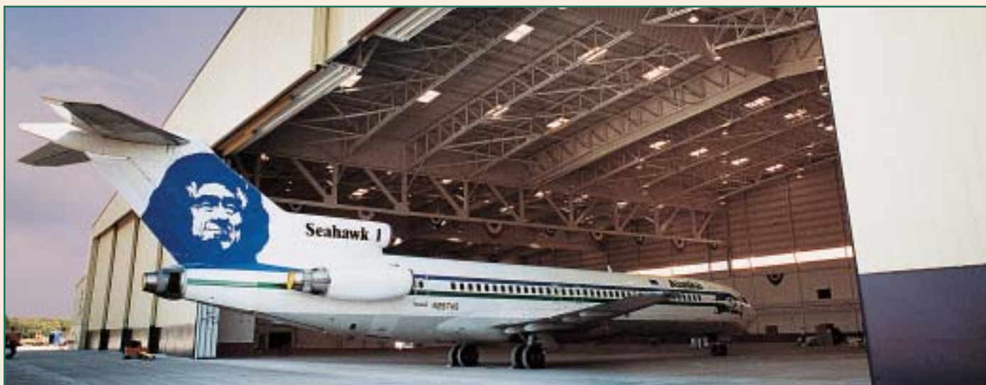
100 SERIES DOORS: Tramco Corporation's maintenance facility at Everett, Washington fills their 538'-0" wide by 50'-0" high door opening with 2 sets of 4-leaf and 2 sets of 5-leaf Fleming Motor Operated Full FLOATING GROUP Hangar Doors. Each group of doors is interconnected with a WRAP-AROUND CABLE SYSTEM. The hangar door system also incorporates a 15'-0" wide by 20'-0" ROLLING SHUTTER TAIL DOOR.
