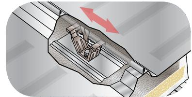
All the performance of the MR-24 Roof System with the addition of insulation and a metal liner.
