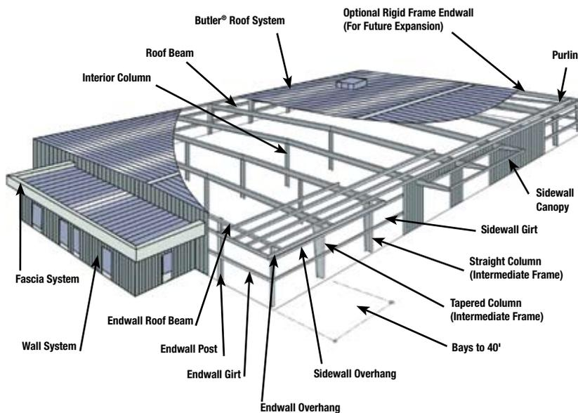
The Widespan system features exclusive factory-punched components—precision engineering that ensures problem-free on-site assembly.
