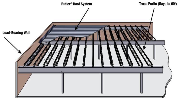
Truss purlin design allows for maximum column-free space.
