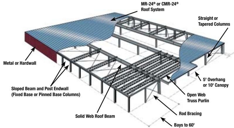
The Landmark 2000 system maximizes interior space with bays of up to 60 feet.
