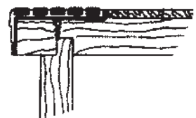
Type 142 Supergrit® attached to wood tread and backed with tile, carpet, or other material.
