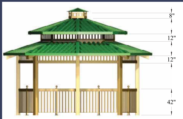
18" wide standing seam panel • galvalume steel, ASTM A792 Gr 50
