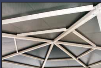
Insulated sandwich panel 3" thick x 48" wide, high density polystyrene between two layers of white stucco embossed .032 aluminum.
