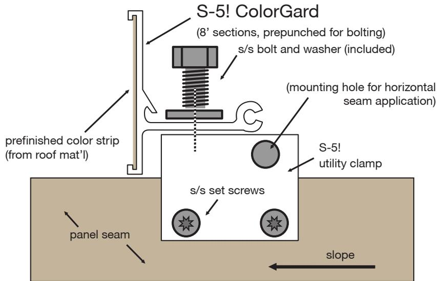
Petersen Aluminum Corporation is stocking the patented ColorGard Snow Retention System. ColorGard is the only product available which will perfectly match the color of the roof. ColorGard achieves this by utilizing a strip of the actual roof material, which is then mounted directly into ColorGard for a perfect match. This strip can be cut in the field or at our factory. An architectural alternative to ColorGard is SnoFence, which uses posts and continuous rods.
