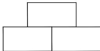
Staggered Butt Joints All Side Joints must occur on Main Tees
