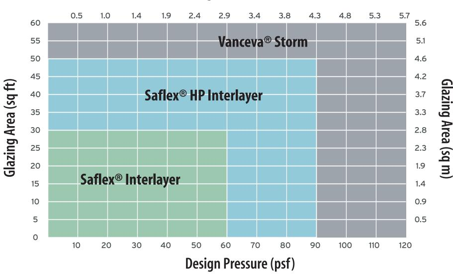
Note: Experienced product performance. Based on panels glazed with structural silicone, minimum 12 mm (1/2 in) glass bite; standard test temperatures 15 - 35 degrees C (59 - 95 degrees F). Not guaranteed for all samples.
