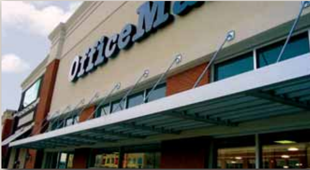
LUMISHADE mapes.com/lumishade High load roll-form hanger rod canopy • Modular design for ease of installation • Loads exceeding 120 PSF • Projections up to 10'
