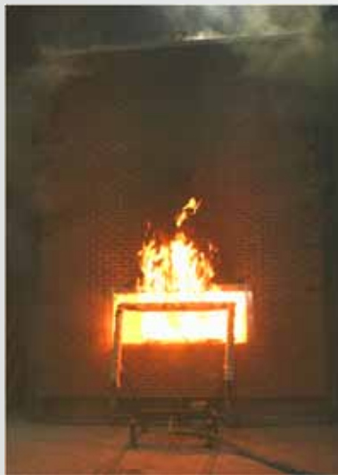
Fire emitting from the NFPA 285 test window.
