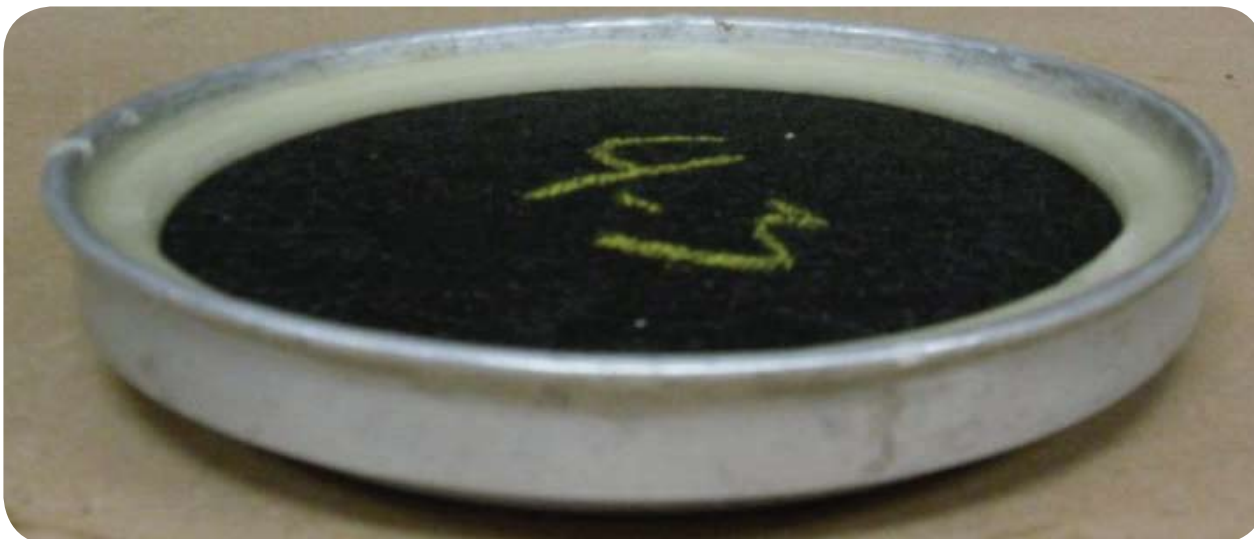
Figure 2: #15 Felt Underlayment Sample–ASTM E 96–6" dia. “Dry Cup”
